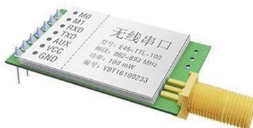
E45-TTL-100 is a 100mW wireless transceiver module with LoRa spread-spectrum technology, operates at 862~893MHz (Default: 868MHz), based on originally imported RFIC SX1276 from SEMTECH, transparent transmission is available, TTL level.
