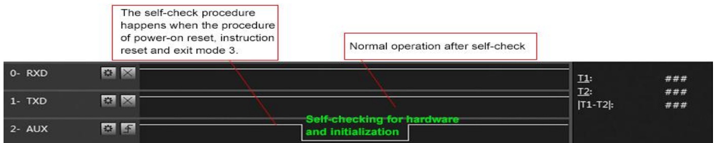
Timing Sequence Diagram of AUX when self-check
